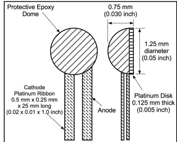
1. Mounting area should be prepared and cleaned with a solvent such as Acetone followed by an Isopropyl Alcohol rinse. Allow time for the solvents to evaporate before sensor mounting.
