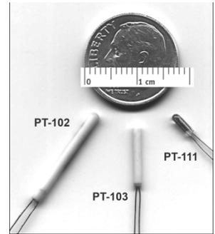
There are three aspects of using a cryogenic temperature sensor which are critical to its optimum performance: 1) proper mounting of the sensor package, 2) proper joining of sensor lead wires and connecting wires, and 3) proper thermal anchoring of the connecting wires. Although the sequence in which these concerns should be addressed is not fixed, all elements covered under each aspect should be adhered to for maximum operating capabilities of the sensor.
