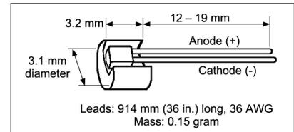
**NOTE:** It is important that no electrically conductive particles lodge between the adapter and sensor. There is a thin braze joint around the sides of the SD sensor and is electrically connected to the sensing element. Contact to the sides with any electrically conductive material will cause a short.
