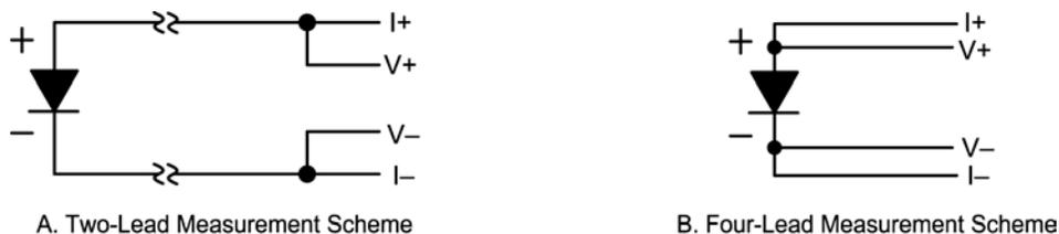
**Figure 1. Two-Lead Versus Four-Lead Measurements**
