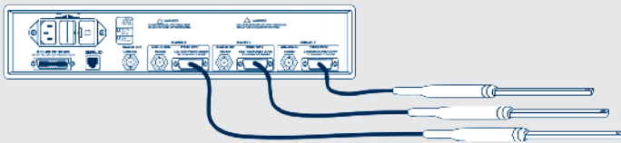
Model 460 configured as 3 separate gaussmeters
